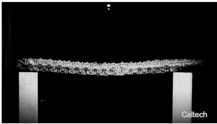
Testing the impact resistance of the material when unjammed (soft). Credit: Caltech
