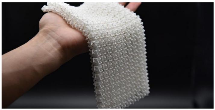
Engineers have developed a material inspired by chain mail that can transform from a foldable, fluid-like state into specific solid shapes under pressure. Credit: Caltech
