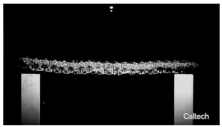
Testing the impact resistance of the material when jammed (rigid). Credit: Caltech
